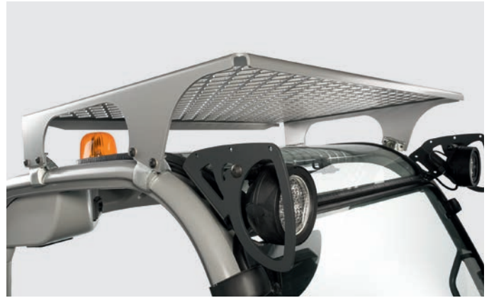
Additional protective grille roof
