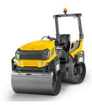
The ergonomic work platform is designed for reduced vibration. The low vibration, easy access and operability of all control elements increase working comfort, operator satisfaction and operator health.
