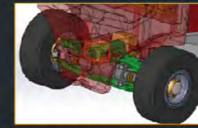
High rotation point steering axle
