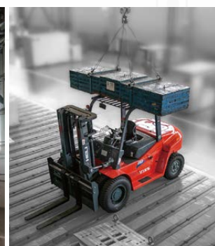
Impact test of overhead guard
