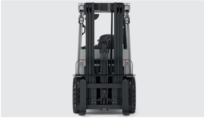
A conveniently positioned mast and a slightly offset operator's seat ensure good visibility
