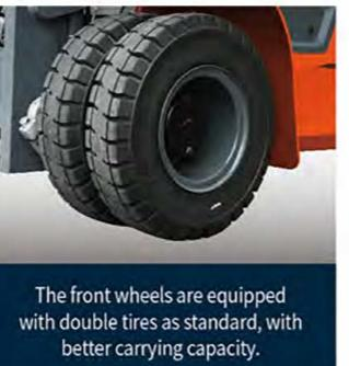
The front wheels are equipped with double tires as standard, with better carrying capacity.
