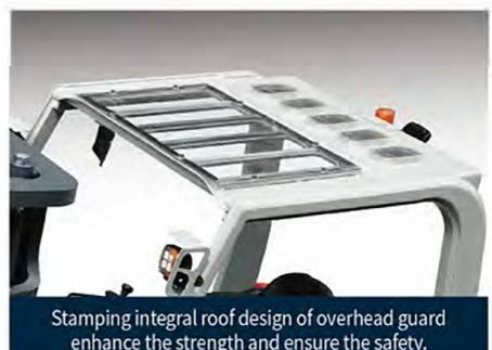
Stamping integral roof design of overhead guard enhance the strength and ensure the safety.
