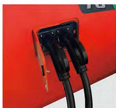
Lithium battery forklift truck is equipped with double gun charging as standard, which greatly reduces the charging time. Lithium batteries have high-density capability and can be used and charged at any time to realize efficient and continuous operation all day long.
